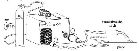
**Attention!** In the most general case, carbon dioxide "CO2" is used as shielding gas for welding of ferrous metals, and aluminium is welded only using inert gases, such as argon "Ar" and sometimes expensive helium "He". As an alternative option for stainless and high-alloy steels, mixtures with different ratios are often used, such as "80%Ar+20%CO2". Other gases can only be used upon approval of the equipment manufacturer.
